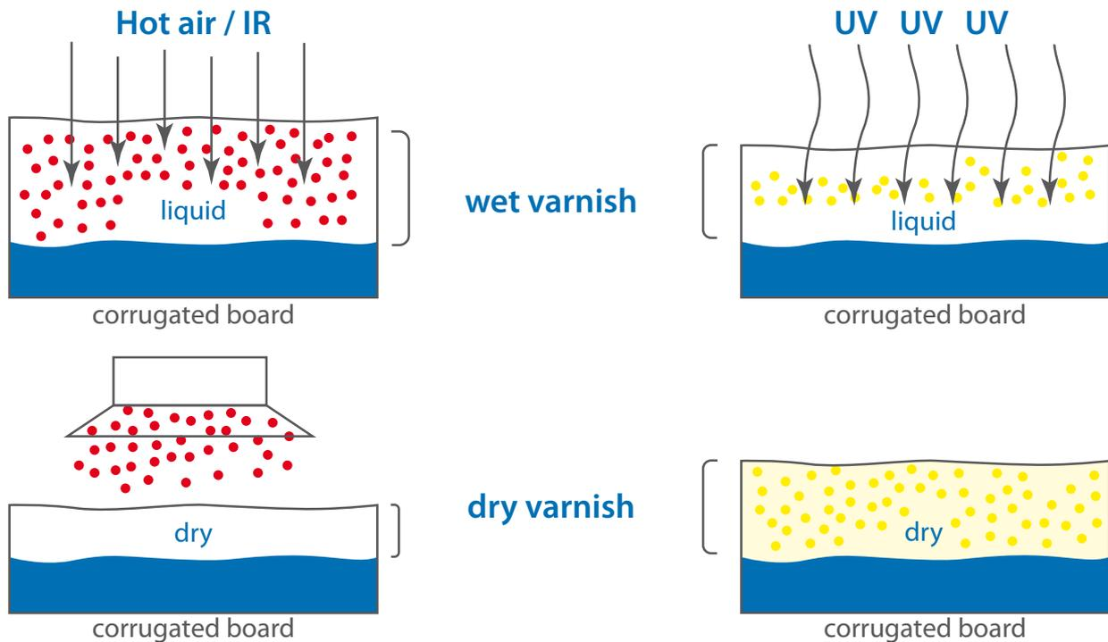
// With conventional drying, the liquid in the coating is evaporated by warm air or infra-red energy. The dry film thickness is thinner than the wet coating thickness.
